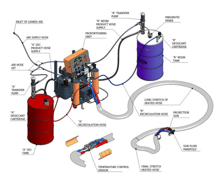
Figure 1. Typical Installation in a G-50 H with recirculation.
