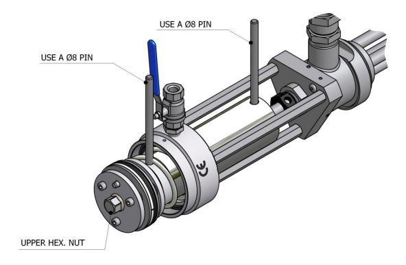
**WARNING!** Do not use the hexagonal geometry of the upper nut of the plunger to loosen and unscrew the rod as this can cause irreparable damage to the plunger interior mechanism.
