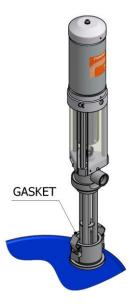
2. Screw the 1/4"NPT-1/4"BSP thread adapter and the ball valve on to the pump, placing sealing paste or teflon tape on the threads to ensure that the unit is properly sealed. Make sure that the ball valve is closed. Do not connect the network air supply yet.
