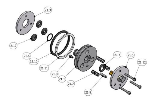
Figure 7. Details of Diagram of Upper Plunger (Pneumatic).
