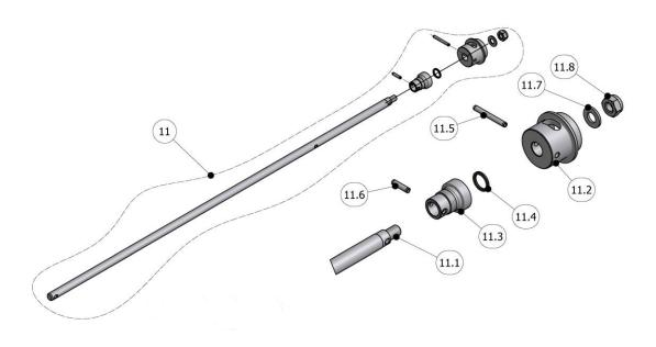
Figure 8. Details of Diagram of Lower Plunger.
